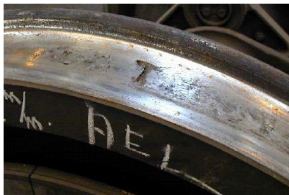
Figure 16c) — Shelling in the centre of a local tread collapse
