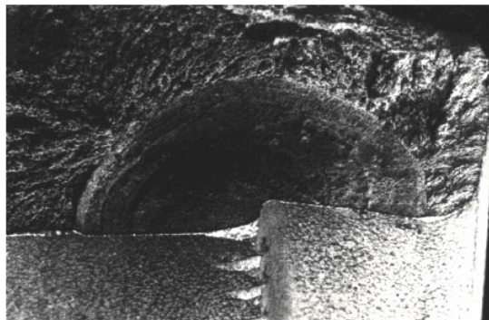
b) Evolution of a fatigue crack initiated on a tooling mark
